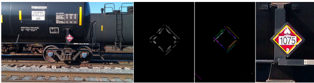
Fig. 1: First method (left to right): original image, segments at \pm 45^\circ , grouped segments, optimal bounding box.
