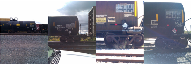
Fig. 5: Samples from the image dataset. From left to right: low resolution, projective distortion, blurred sign, shaded sign.
