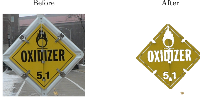
Figure 2. Before and after applying the luminance and chroma thresholds. ( 0.2 < Y < 0.8, c > 0.1 )
