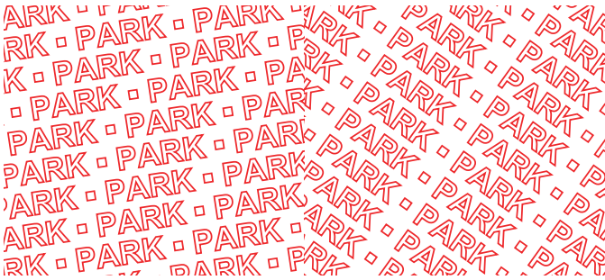
Fig. 5. Varying text orientation to distinguish between adjacent regions; useful if the regions have no other distinguishing graphical attributes.
